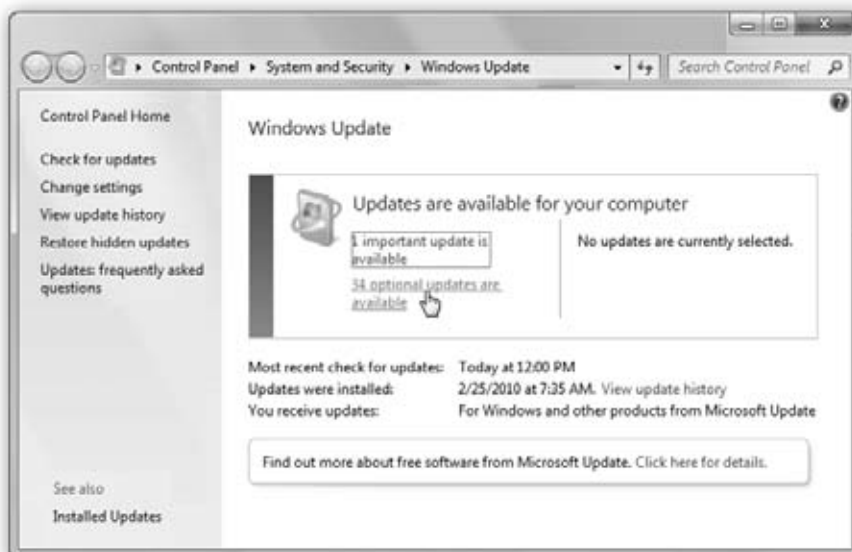
Figure 20-12: If there are any available updates, you can install them by clicking “Install updates.” To get details about an update, click “View available updates.”
