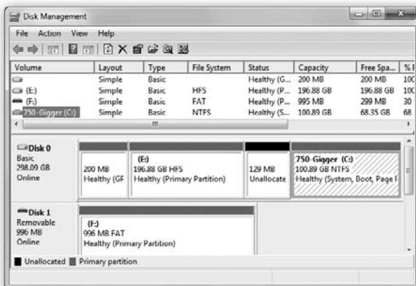
Figure 21-1: The Disk Management console is the central toolbox for all your disk-related tasks. This is where you create the dynamic volumes on your disks. Notice that drive E: is in trouble—it has no remaining free space. Read on for the solution.
