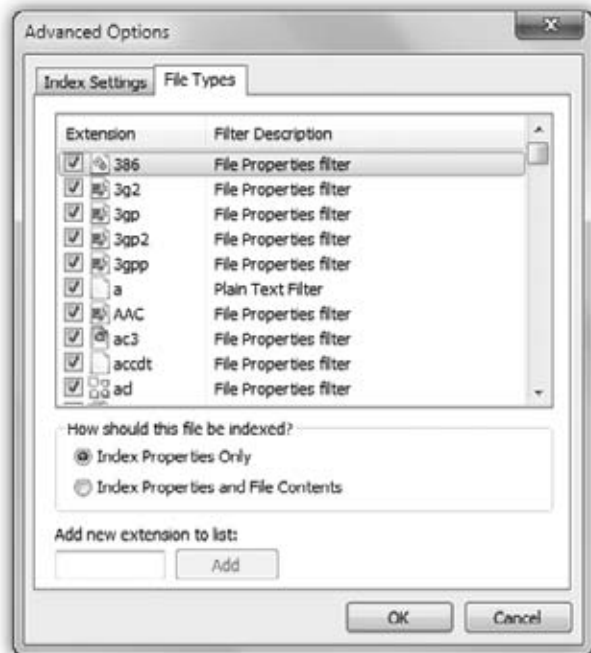
Figure 3-6: Using the “How should this file be indexed” options at the bottom of the box, you can also make Windows stop searching these files’ contents—the text within them—for better speed and a smaller index.
