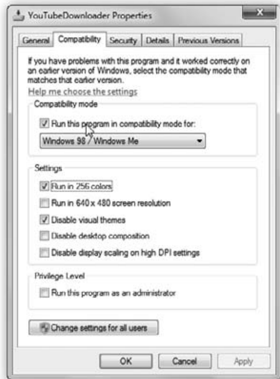
Figure 6-21: By turning on "Run this program in compatibility mode for" and choosing the name of a previous version of Windows from the list, you can fool that program into thinking it's running on Windows 95, Windows Me, Windows NT, or whatever.
