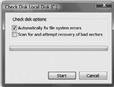
Figure 20-3: Checking your disk for errors regularly will go a long way toward making sure your files won't get corrupted. If you use the "fix file errors" option, the check occurs at the next startup; the "scan" option goes into effect immediately.
