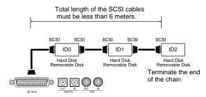
Be sure to attach (or switch on) the terminator for the last drive in the chain. If more than one external drive is connected, make sure that the total length of the cable does not exceed 6 meters. (For details on connections, refer to the owner's manual for your external drive.)
