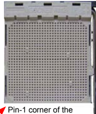
Pin-1 corner of the CPU socket
