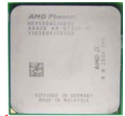
Pin-1 triangle marking of CPU
